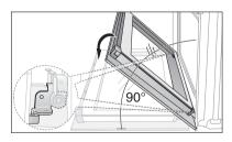
**2.** Undo the **clamping levers** (A) on both door hinges **fully**.
